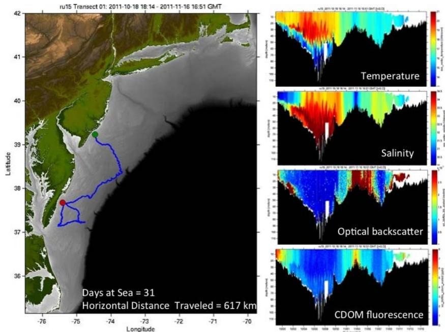
**Figure 6.** The MARACOOS glider mission conducted in October 2011. The measurements toward the end of this longer-than-normal mission were degraded because of the rapidly decreasing battery power.
