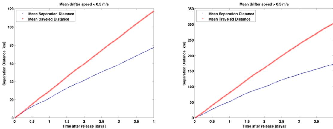
**Figure 1.** Simulated separation distance (blue) compared to persistence (red) as a function of time for four-day period. Drifters with mean speed less (more) than 0.5 m/s are presented in the left (right) panel.
